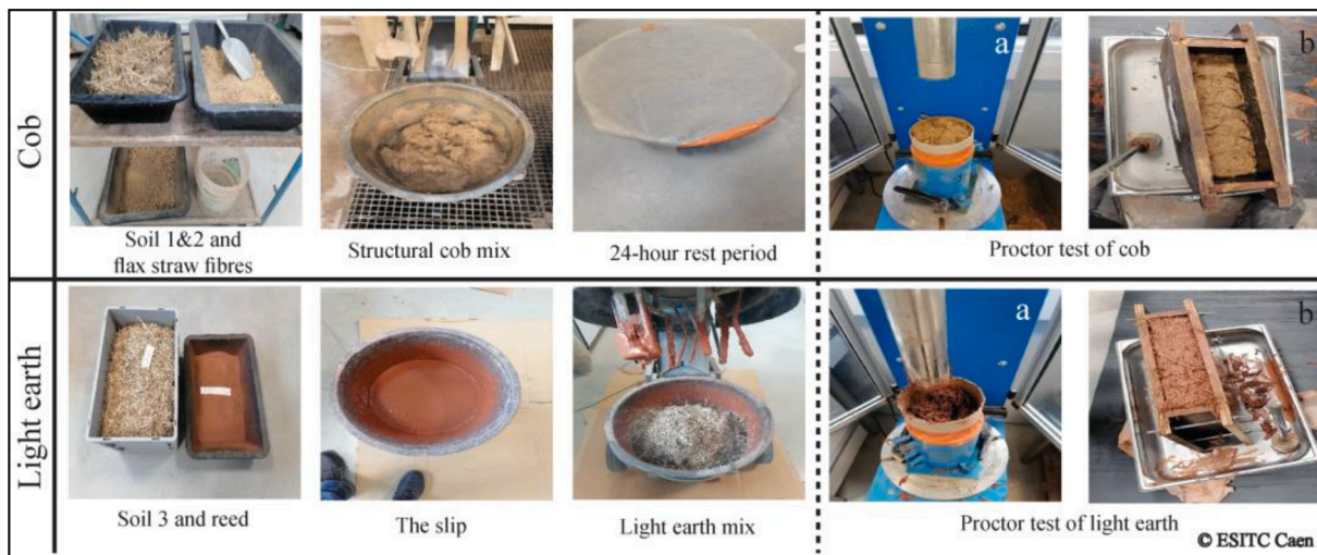
Fig. 5. Preparation of cob and light earth specimens in the laboratory: (a) cylindrical specimens for compressive strength tests and (b) prismatic specimens for thermal conductivity tests.
