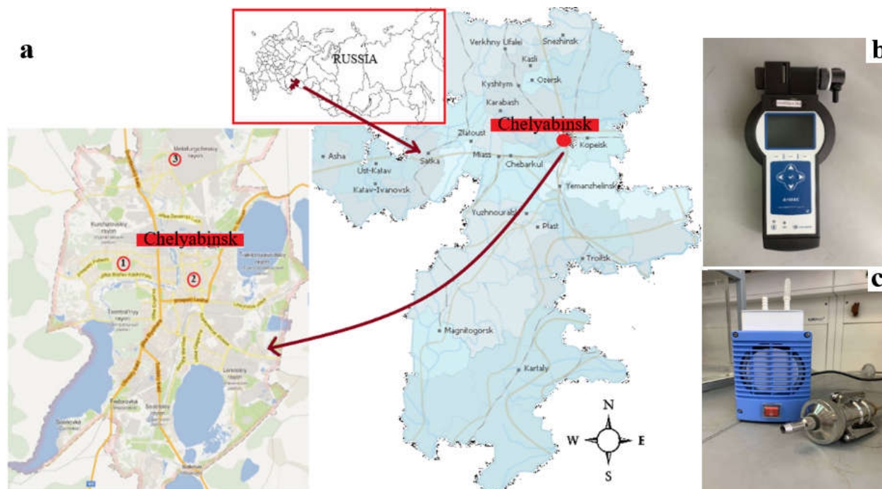
Figure 1. The area under study and the observation instruments used to record data. (a) Chelyabinsk (Russia) and the location of the three sampling stations. (b) Atmos (NTM Protection, Moscow, Russia) device, providing simultaneous measurement of the hourly data of PM 2.5 and PM 10 . (c) The aerosol cascade impactor sampler.
