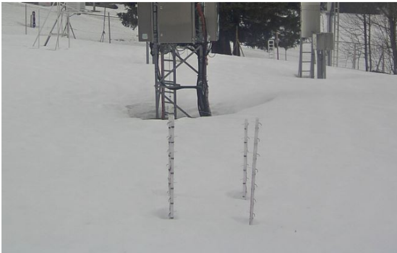
Fig. 9. Meteo France webcam image from midday on 12th April showing preferential melting has created cavities around the poles, exposing more electrodes than might be expected from the observed snow depth.
