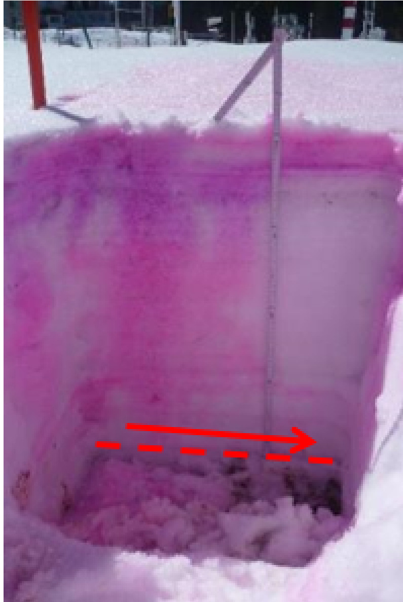
Fig. 7. Dye tracing experiment carried out on 20th March 2019. The density contrast, along which horizontal flow occurred, is marked.
