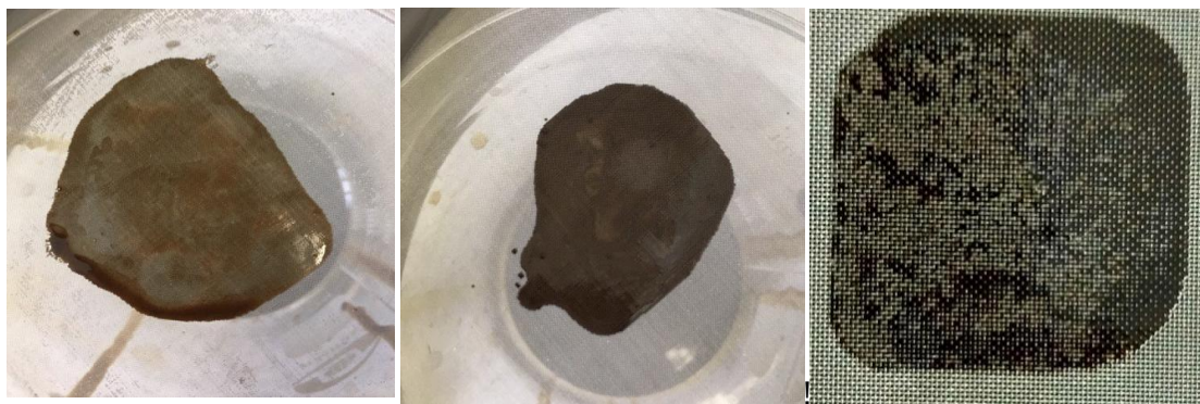
507 508 Figure 6. The results of filtration of Emulsion A mixed with crude oil through a 100- 509 mesh sieve that corresponds to approximately 150 \mu\text{m} diameter pores. The left picture 510 shows that the mixture of crude oil with Emulsion A retains properties of a single- 511 phase fluid capable of flowing through 150 \mu\text{m} pores of the reservoir. The middle and 512 right picture show no residues on the filter after flowing the mixture of Emulsion A 513 and crude oil.
