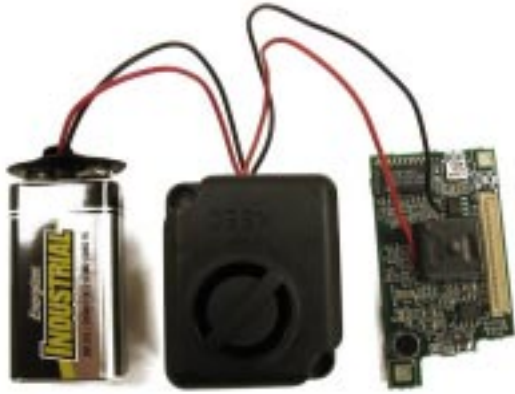
(a) Extended sensor board with 9V battery
