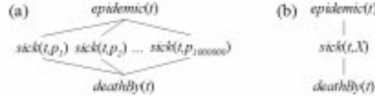
Figure 1: Computing an answer to query P(\text{deathBy}(t)|\text{epidemic}(t)) from our example with a single disease typhus ( t ) and a million people will be expensive for the propositional grounded model (a) as it has a large tree-width, but cheap for the lifted model (b) since it is a linear graph.
