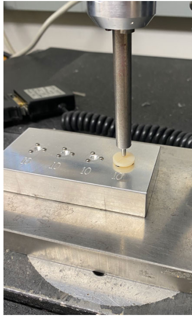
Figure 17: Disk Specimen Set-Up on the Universal Testing Machine
