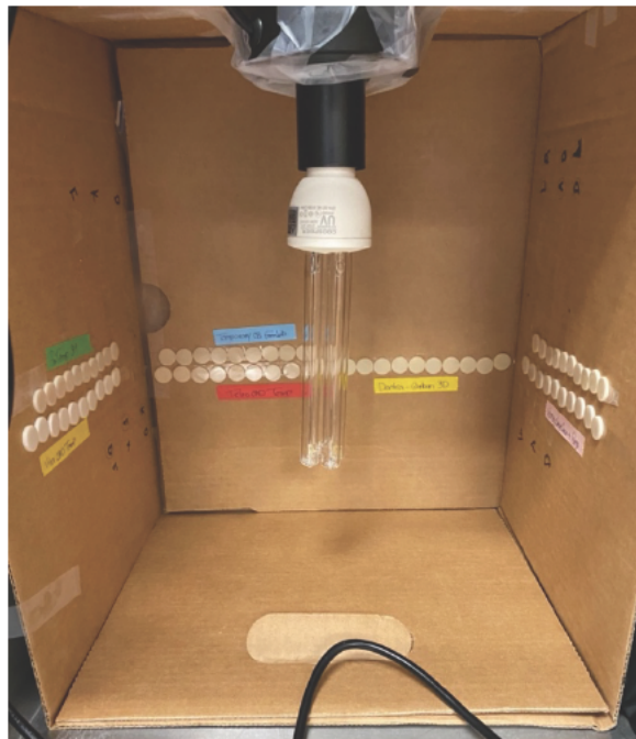
Figure 21: UVC Light Treatment Apparatus and Set-Up
