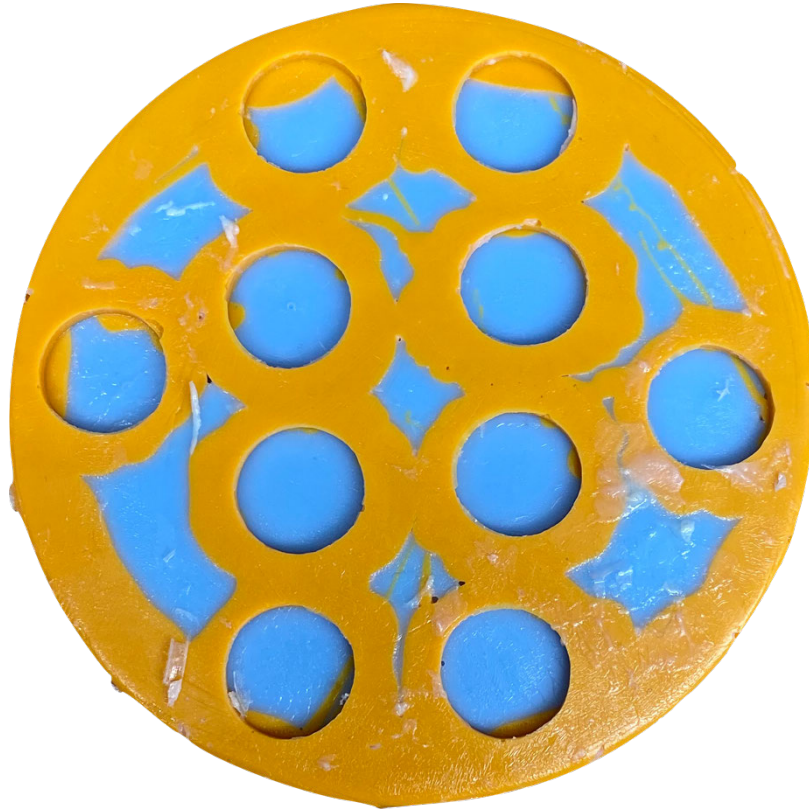
Figure 8: Custom Silicone mold utilized to fabricate conventionally prepared disk specimens
