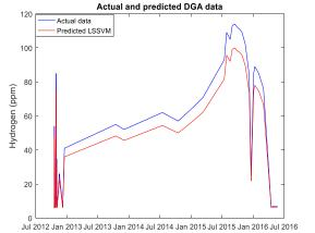
Figure 5 Actual and predicted DGA data using LSSVM model - hydrogen
