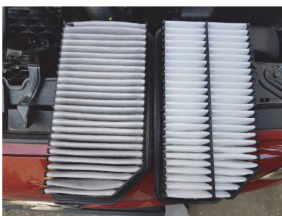
Figure 28 Old (left) and new (right) air filter
