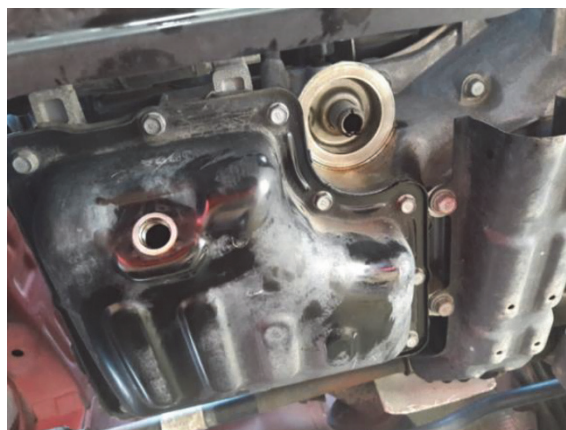
Figure 24 Removed oil drain plug and oil filter
