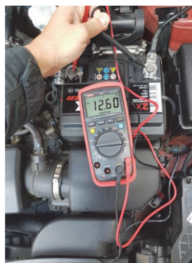
Figure 30 Checking the battery charge status
