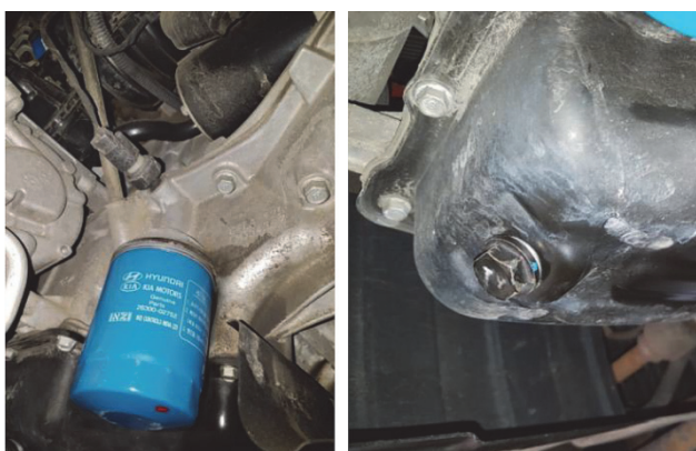
Figure 27 Looking for oil leaks after filling the engine with new oil
