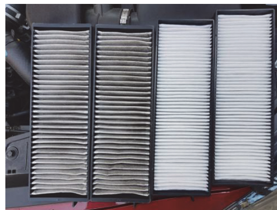
Figure 29 Passenger compartment (air conditioning) filter used left and new right
