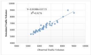
Figure 5 Comparison of field and simulated traffic volume
