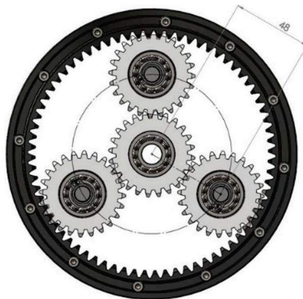
Figure 5 Inside gears of planetary gearbox
