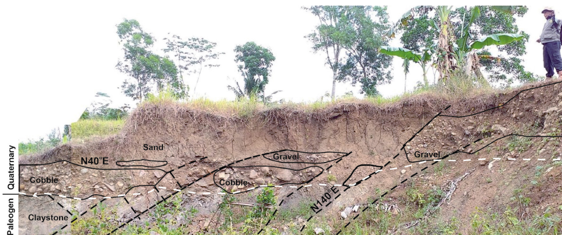
Figure 15: Outcrop of river terrace above the claystone bedrock of the Karangsambung Formation.
