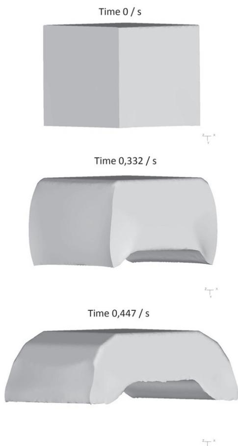
**Figure 4** Simulation results of pre-forging process
