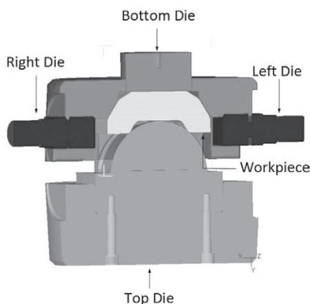
**Figure 3** 3D geometric model of final forging sequence
