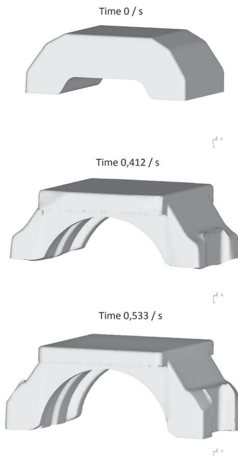
**Figure 5** Simulation results of final forging process
