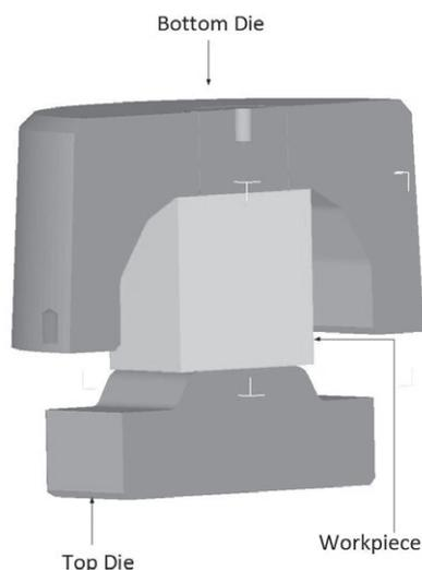
**Figure 2** 3D geometric model of pre-forging process
