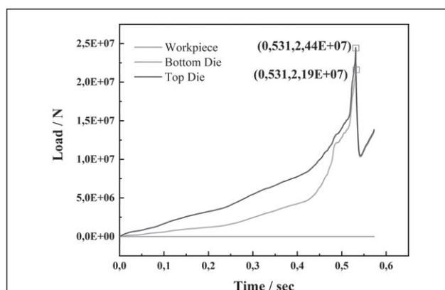
**Figure 6** Load-stroke curve in forming
