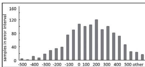
Figure 2 Histogram of rolling force error of rolling mill
