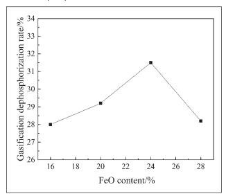
Figure 4 Effect of FeO content on the gasification dephosphorization rate
