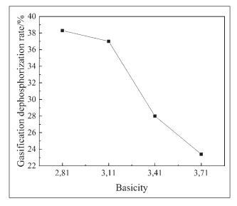
Figure 3 Effect of binary basicity on the gasification dephosphorization rate
