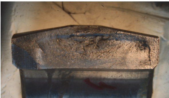
Figure 30 Case crushing-induced fracture of the roller specimen, loading 15000 N
