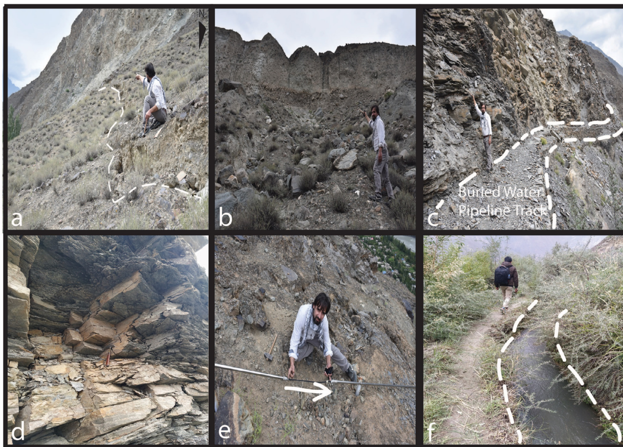
Figure 4: Field photographs of the Mayoan landslide, (a) surface cracks on the top eastern part of the landslide, (b) glacial scree deposits on the top eastern part of the landslide, (c) highly sheared deformed bedrock exposed along the buried water pipeline track, (d) fractures within the deformed bedrock exposed at the surface (e) extensometer showing the movement in the central part of the landslide, (f) open water channel along the eastern part of the landslide
