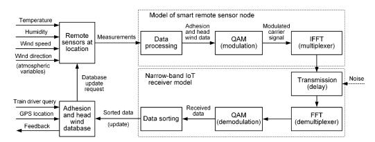
Figure 7. Block diagram representation of NB IoT remote sensor node connection to central track adhesion and head wind database
