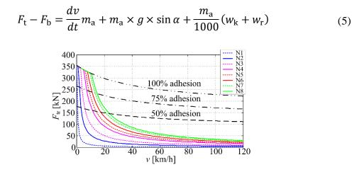
Figure 5. Maximum traction force vs. velocity curves with 'Notch' command and wheel-to-track adhesion as parameters
