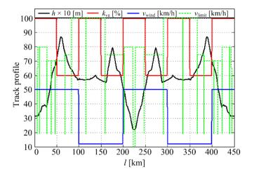
Figure 2. Altitude, traction coefficient, head wind speed, and train speed limit profiles for the rail route considered in this work
