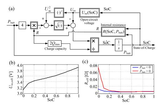
Figure 6. Battery power flow model (a); cell open-circuit voltage vs. SoC (b) and cell internal resistance vs. SoC and current sign (c)
