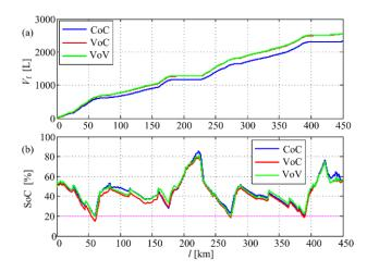
Figure 11. Comparative cumulative fuel consumption of locomotive (a) and SoC variable (b)
