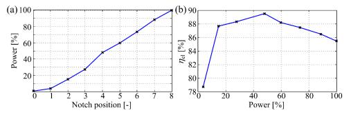
Figure 4. Locomotive power production vs. 'Notch' command (a) and overall electric power conversion efficiency curve (b) [43]
