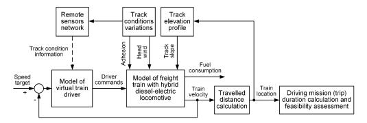
Figure 1. Principal block diagram (flowchart) of proposed methodology for railway train fuel efficiency and safety assessment
