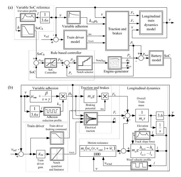
Figure 3. Block diagram of battery-hybrid locomotive model (a) and electrical traction sub-model (b)
