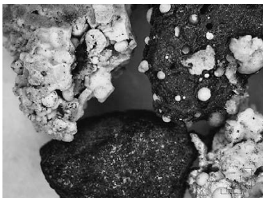
Figure 2 Lumpy aggregates of mineral phases of various compositions in a coarse fraction estimate of alumina
