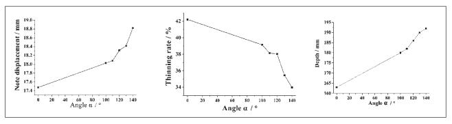
Figure 7 Influence of a on forming quality. (a) Displacement of node flow (b) Thinning rate (c) Drawing depth
