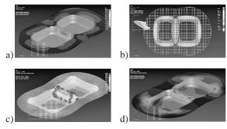
Figure 3 Simulation of drawing process (a) Thinning rate of blank (b) Material displacement (c) Strain vector (d) Maximum strain
