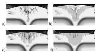
**Figure 6** Influence of guiding groove depth on forming quality (a) h = 20 mm (b) h = 10 mm (c) h = 5 mm (d) h = 1 mm
