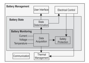
Fig. 4 Illustration of a battery management system - BMS
