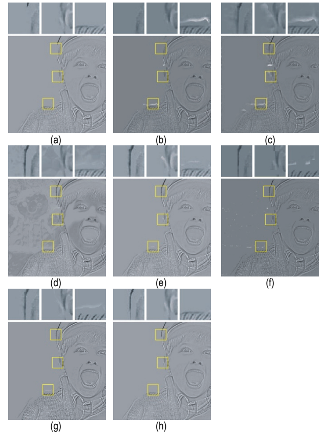
Figure 9 Difference of fused image and far focused "Joy" source images, a) QMIF [13]; b) DCT [25]; c) DWT [23]; d) GFF [24]; e) DSIFT [18]; f) DCT-EoL [3]; g) TSF [26] and h) Proposed
