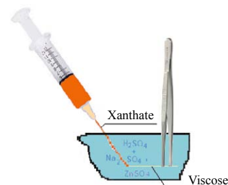
Fig.2 Scheme of viscose wet spinning by pressing xanthate through a hypodermic needle into a spinning bath
