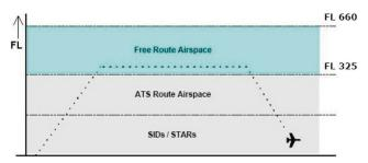
Fig. 2. Illustration of the FRA in Croatia and its relationship to ATS-governed airspace. Adapted from ref. [6]
