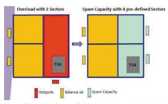
Fig. 6. Illustration of sector division during increased workload. Adapted from ref. [18]
