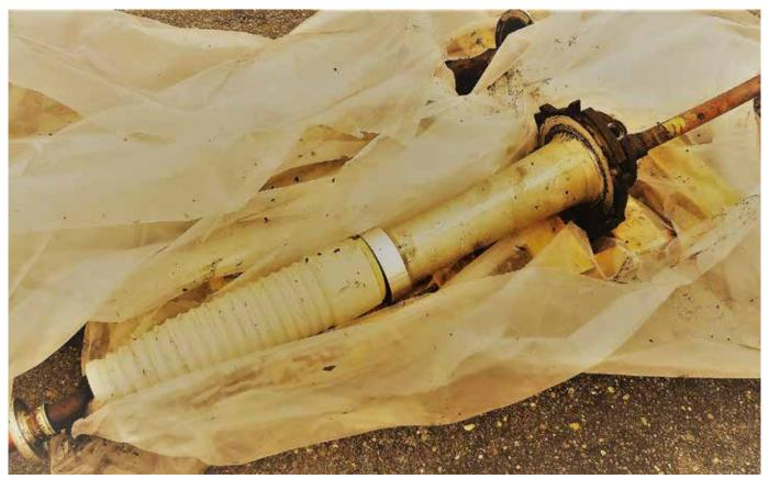
Figure 3. Investigated ABB, 69 kV, type O+C bushing failure for case study 2
