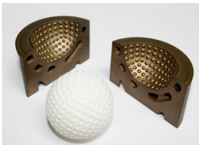
Figure 3 Hard metal mould insert [6]
