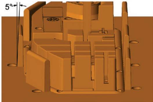
Figure 8 Increased draft angles [5]
