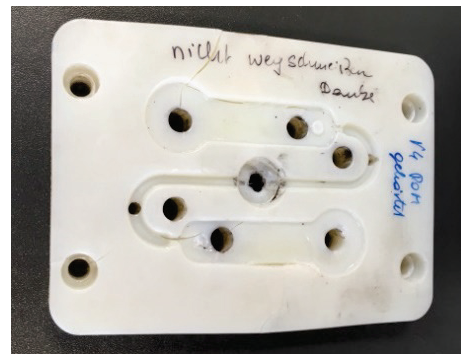
Figure 18 PolyJet mould plate with cracks [14]
