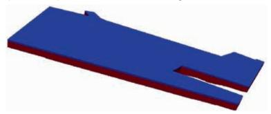
Figure 5: Distribution of water and air within the domain (red region is the water phase while blue is air)
