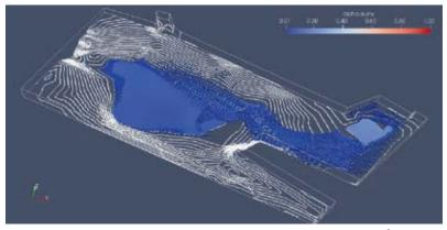
Figure 9: Sediment deposition area at a flow rate of 70 m³/s
