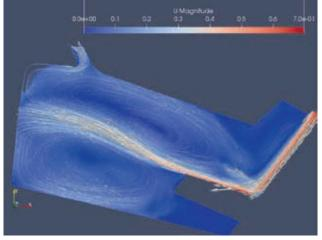
Figure 12: Velocity field at a flow rate of 70 m<sup>3</sup>/s
