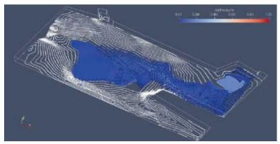
Figure 8: Sediment deposition area at a flow rate of 35 m<sup>3</sup>/s
