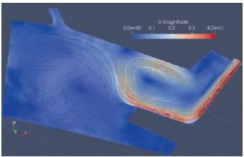
Figure 6: Velocity field at a flow rate of 35 m<sup>3</sup>/s
