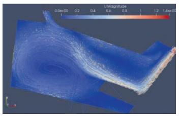
Figure 7: Velocity field at a flow rate of 70 m<sup>3</sup>/s
