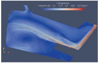
Figure 11: Velocity field at a flow rate of 35 m<sup>3</sup>/s
