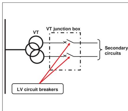
Figure 8. Voltage transformer junction box
