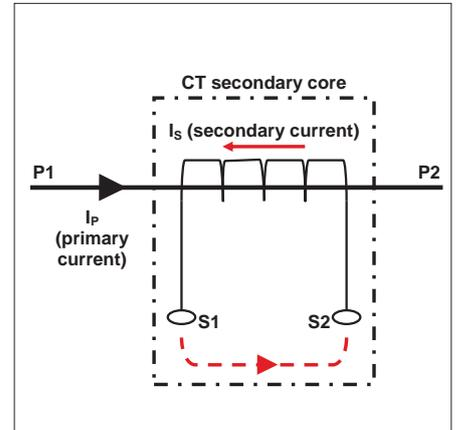
Figure 9. Current transformer connection
