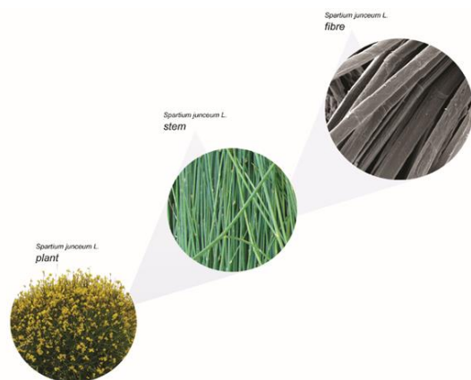
Figure 1. Representation of SJL plant and its structural above ground axis, which is raw material for fibre production; Left to right: SJL shrub during bloom; Freshly harvested SJL stem; Scanning electron micrograph of SJL fibres extracted from the SJL stem [1]
