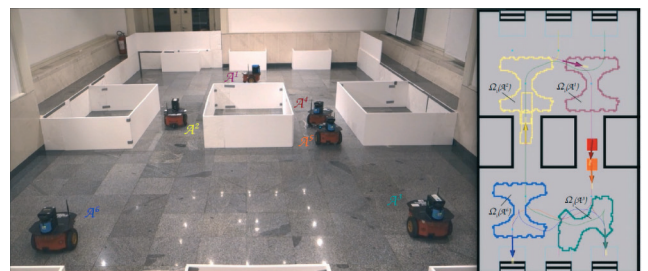
Fig. 6. Validation of the algorithm performance on a system composed of six Pioneer 3DX robots in a laboratory environment with terminals and corridors. [23].
