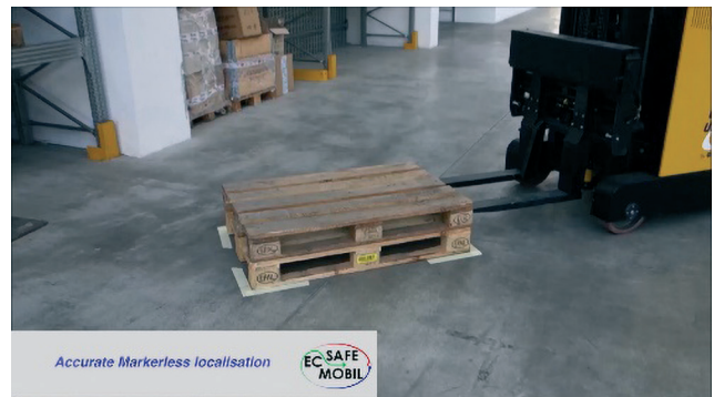
Fig. 2. Markerless pallet delivery of an AGV in the industrial facility with the localization accuracy <0.01\text{m} , 0.5^\circ provided by the AMCL+ICP+FFT localization algorithm stack [20].
