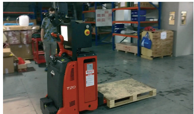
Fig. 10. Tests with a Linde T20 autonomous forklift in RV Automation facility in Hong Kong during execution of a pallet delivery task.
