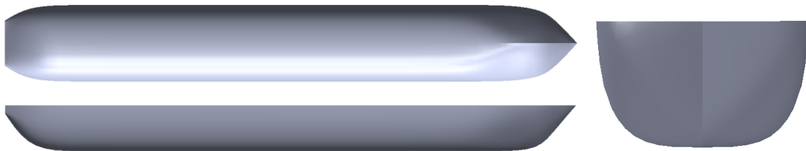
Fig. 8. Profile of the icebreaking tanker - MT Uikku
