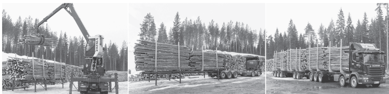
Fig. 1 Transshipment of pulpwood from regular trucks and terminal stock onto an HCT truck (5+5 axle full trailer, 84 t gross weight) equipped with a demountable truck body. Photo: Esa Hirvonen
