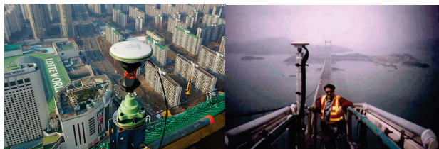
Figure 3 GPS monitoring antennas on a skyscraper [18] and bridge [19]
