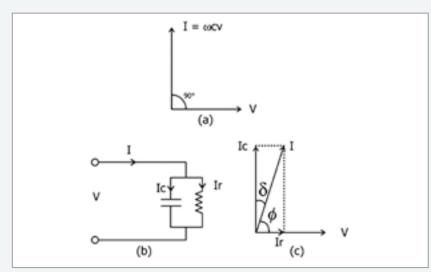
Figure 6. The loss angle  $\delta$  = 90 -  $\phi$  is the angle between the phasors  $I_c$  and I
