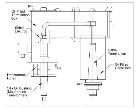
Figure 7b. Oil-to-oil type bushing used for cable connection through an oil-filled cable box
