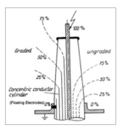
Figure 3. Comparison of potential distribution in graded and ungraded bushings [5]
