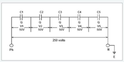
Figure 1. A specimen circuit of capacitors, each of 20 nF, connected in series
