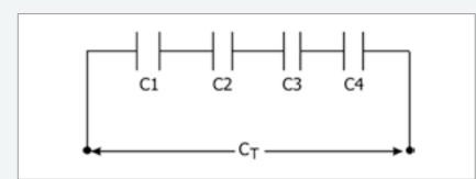
Figure 5. Equal capacitors in series
