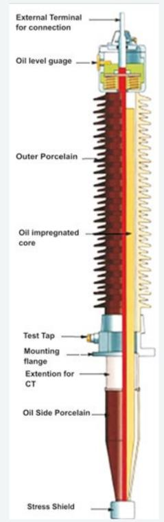
Figure 7a. Components of a condenser bushing [7]
