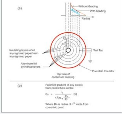
Figure 2. (a) The concept of potential graded condenser bushings [3]; (b) calculation of the potential gradient  $E_x$  at a distance x from the centre of the cylindrical tube/rod of the bushing [4]
