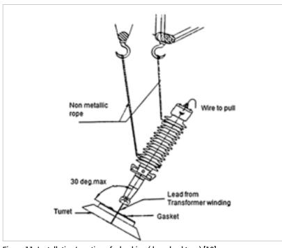
Figure 11. Installation/erection of a bushing (draw-lead type) [10]
