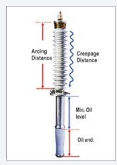
Figure 9. Arcing distance and creepage distance of the bushing
