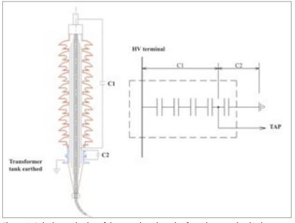
Figure 4.  $C_1$  is the total value of the capacitors in series from the central rod/tube to test tap and  $C_2$  is the total value of capacitors from test tap to the bushing flange
