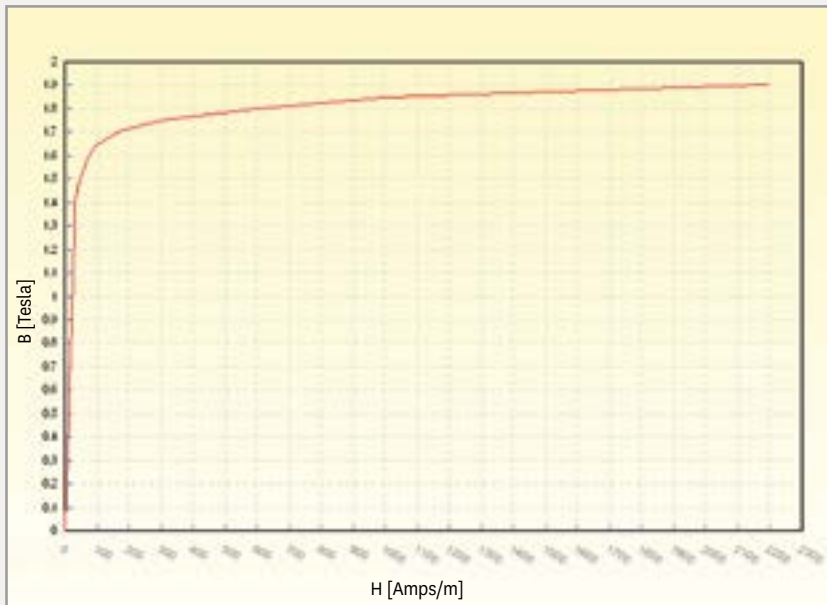
Figure 3. Basic magnetization curve of the magnetic steel 2212
