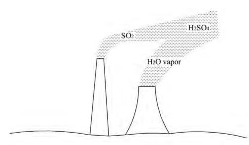
**Figure 1.** Schematic diagram of stack and cooling tower plume mergence **Slika 1.** Shematski dijagram miješanja perjanica iz dimnjaka i hladnjaka.
