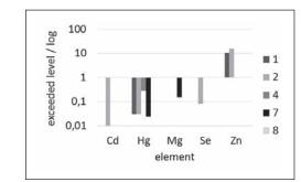
Figure 1 Permissible levels exceeded for inert waste based on water extracts of the dust types subject to tests
