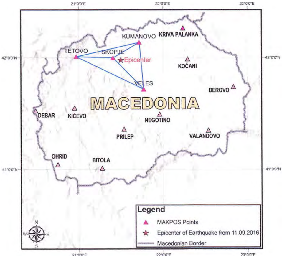
Figure 1. GNSS reference stations of the MAKPOS network and the net for determination shifts of the Earth’s crust before and after the earthquake in Skopje in 2016.
