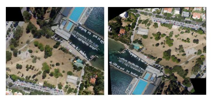
Fig. 3. Image mosaic of the area of interest before (left) and after (right) applying world file transformation
