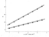
Fig. 5. Determination of complex composition by slope-ratio method at pH = 1.0. Concn. HX 5×10<sup>-4</sup> M, concn. Fe (III) is varied,  $\lambda = 570$  nm ( $\bigcirc$ ) and 470 nm ( $\square$ ). Cocn. Fe (III),  $5 \times 10^{-4}$  M, concn. HX is varied,  $\lambda = 570$  nm ( $\textcircled{\bullet}$ ) and 4707 nm ( $\blacksquare$ ).
