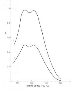
Fig. 8. Absorption spectrum of iron (III)-HX complex in chloroform. Concn. HX  $5 \times 10^{-3}$  M, concn. Fe (III)  $8 \times 10^{-5}$  M (1) and  $1.6 \times 10^{-4}$  M (2).
