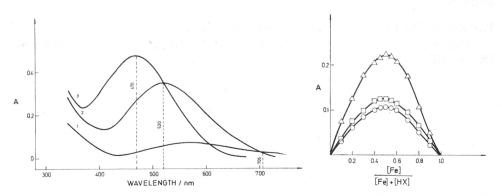
Fig. 1. Absorption spectra of iron (III)-HX complexes in aqueous solution containing 20% ethanol. Concn. Fe (III) :  $1 \times 10^{-4}$  M, concn. HX :  $1 \times 10^{-4}$  M, pH = 1.0 (1), concn. HX :  $2 \times 10^{-4}$  M, pH = 2.5 (2) and concn. HX :  $3 \times 10^{-4}$  M, pH = 4.0 (3).
