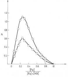
Fig. 9. Determination of complex composition in chloroform by Job's method. [Fe] + [HX] = = 1 × 10<sup>-3</sup> M,  $\lambda$  = 420 nm 470 nm (O) and [Fe] + [HX] = 6 × 10<sup>-4</sup> M,  $\lambda$  = 420 and 470 nm (D).
