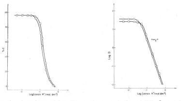
Fig. 6. Extraction dependence of iron (III) on the concentration of HCl (O) and HClO<sub>4</sub> ( $\Box$ ). Concn. Fe (III)  $1 \times 10^{-4}$  M, concn. HX  $5 \times 10^{-3}$  M. Fig. 7. The dependende of distribution ratio, D, of iron (III) on the concentration of HCl (O) and HClO<sub>4</sub> ( $\Box$ ). Concn. Fe (III)  $1 \times 10^{-4}$  M, concn. HX  $5 \times 10^{-3}$  M.
