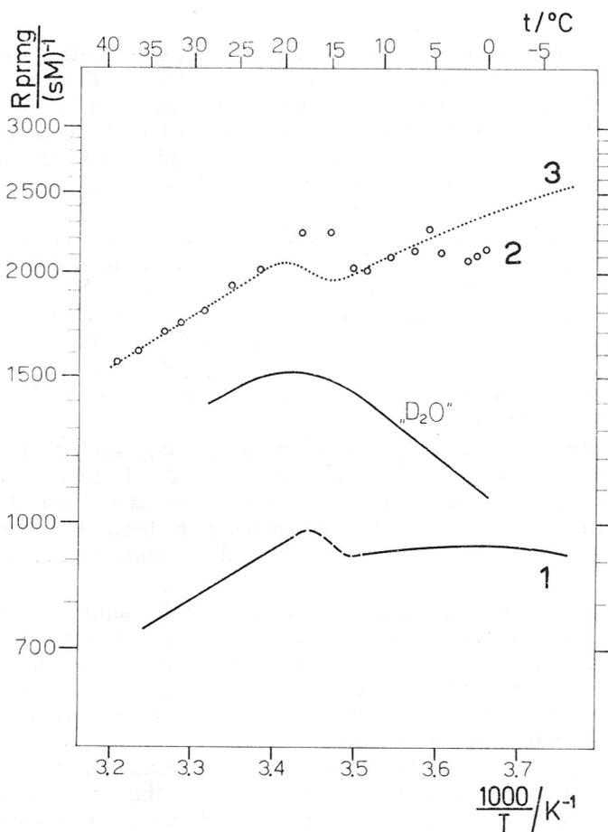
Figure 6. The molar paramagnetically induced relaxation rates derived from Figure 5, with the same numbering of the samples. »D<sub>2</sub>O« indicates similar temperature dependence for the microsomal P-450 prepared in D<sub>2</sub>O, to which 19% H<sub>2</sub>O had been added (the corresponding original and CO-dithionite reduced data are not shown in Figure 5).
