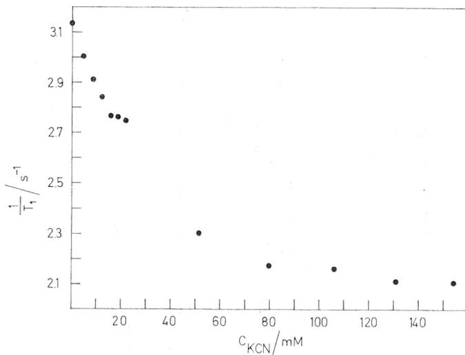
Figure 3. The longitudinal proton magnetic relaxation rates,  $1/T_1$ , (ordinate) of the solubilized cyt P-450 (0.625 mM in P-450 haem, 0.180 mM in P-420 haem, and 0.086 mM in cyt  $b_5$  haem, initial conc.) in dependence on concentration of KCN added (abscissa), at  $24.5 \pm 0.5^\circ C$ .
