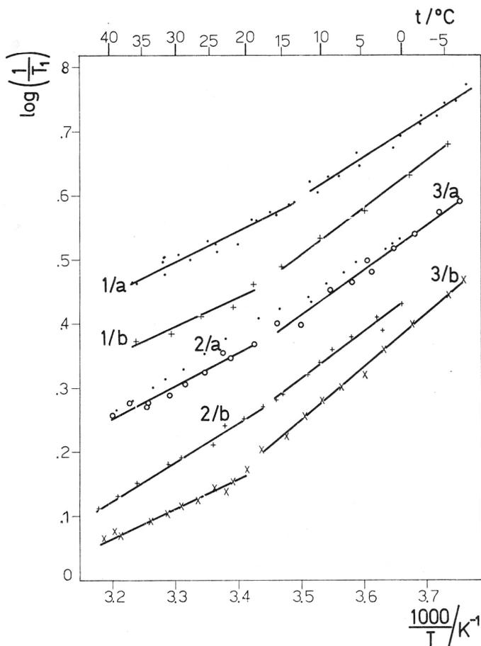
Figure 5. Arrhenius plots for PMR rates of solubilized (1), microsomal (2) and reconstituted (3) P-450 samples. (See text for the corresponding concentrations.) The data for the original samples are designated (a), those for the CO-dithionite reduced (b).
