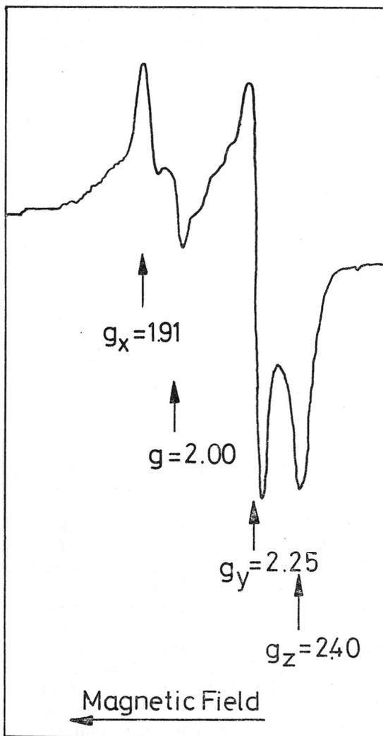
Figure 2. ESR spectrum of cytochrome P-450 from microsomes; temperature 77 K, modul. ampl. 80 Gauss.
