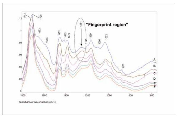
Fig. 14. ATR FTIR spectra of amber finds found in Hungary with the so-called Baltic shoulder around the 1200 cm-1 region ('fingerprint region'). A-653211 (Kötegyán); B-1025 (Budakalász M0/S-12, Grave 1025); C-46194868 (Füzesabony-Öregdomb); D-3195232 (Hernádkak); E-11952188 (Megyaszó, Grave 121); F-11952152 (Megyaszó, Grave 95).
