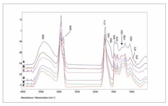
Fig. 13. Amber finds from the Hungarian Bronze Age: ATR FTIR spectra. A-653211 (Kötegyán, depot find, bead); B-1025 (Budakalász M0/S-12, Grave 1025, bead); C-46194868 (Füzesabony-Öreg-domb, settlement layer, bead); D-3195232 (Hernádkak, gravegood, bead); E-11952188 (Megyaszó, Grave 121, bead); F-11952152 (Megyaszó, Grave 95, bead).
