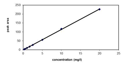
**Figure 3.** Calibration curve of sulfate, the correlation coefficient  $R^2=0.9999$ **Slika 3.** Kalibracijska krivulja sulfata, koeficijent korelacije  $R^2=0.9999$
