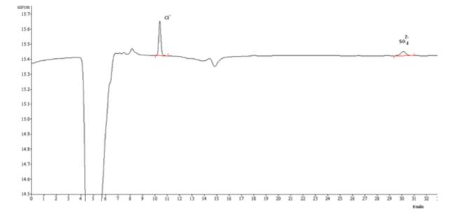
**Figure 4.** Chromatogram of real bio-ethanol sample **Slika 4.** Kromatogram realnog uzorka bio-etanola
