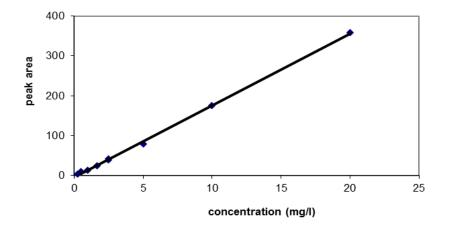
**Figure 2.** Calibration curve of chloride, the correlation coefficient  $R^2=0.9997$ **Slika 2.** Kalibracijska krivulja klorida, koeficijent korelacije  $R^2=0.9997$
