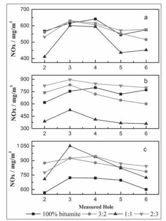
**Figure 2** Variation of the concentration of NOx for each measured hole under different coal ratios and fuel-staged is 15:85. a) Air excess coefficient of 1,4. b) Air excess coefficient of 1,2. c) Air excess coefficient of 1,0.
