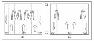
Figure 5 Air flow field from Z1 (measured hole 1) to Z2 (measured hole 4) cross-section
