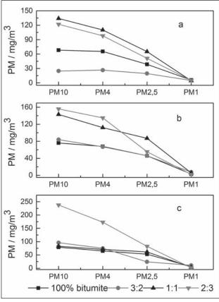
**Figure 4** Particulate matter concentrations under different coal ratios and fuel-staged ratio of 15:85 conditions.
