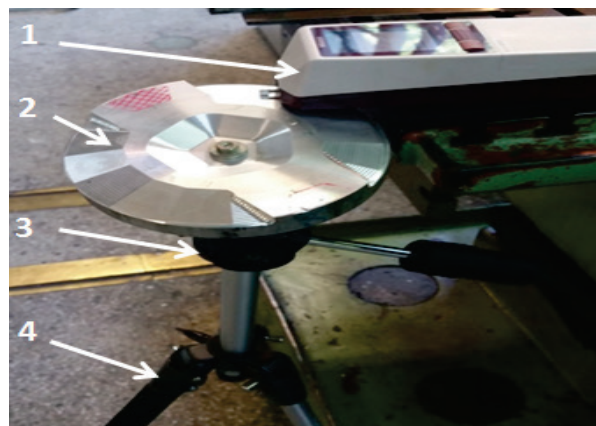
Figure 2 Roughness measurements: 1- MitutoyoSurfTest; 2 - machined part; 3 - alignment device with 3 degrees of freedom; 4 - tripod.
