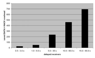
Fig. 9. Carousel scenario – reduced overhead (DATA + NACK) compared to NORM
