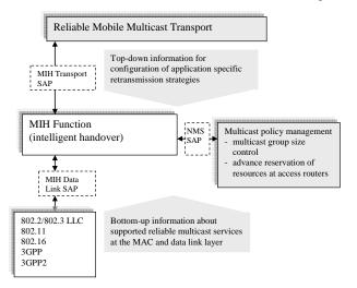
Fig. 3. Usage of IEEE 802.21 MIH for reliable multicast support
