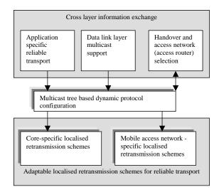
Fig. 2. Cross-layer optimization of reliable mobile multicast transport
