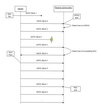
Fig. 4. Retransmission scheme for the reliable carousel multicast
