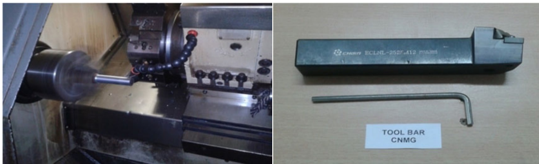
Fig. 3 CNC machine with a tool holder
