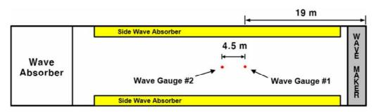
Fig. 11 Wave gauge set-up for calibration and pre-testing
