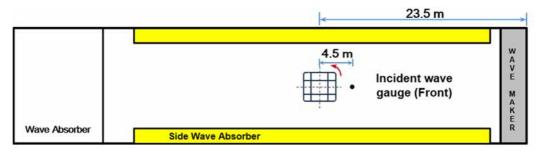
Fig. 5 Sketch of wave gauge position and experimental body
