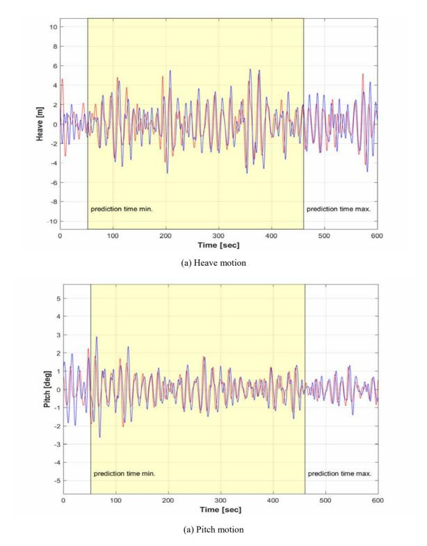
**Fig. 18** Motion prediction based on wave information at gauge position #1 under quartering sea/condition 1/random seed #1 with (a) heave, and (b) pitch motion. The red dashed line depicts the result of motion prediction and the blue dashed line depicts the measured motion.
