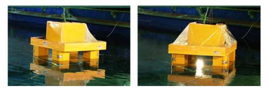
Fig. 7 Model setup (head sea, bow quartering sea)
