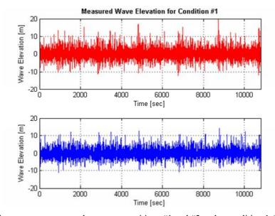
Fig. 12 Time series measurements made at gauge positions #1 and #2 under condition 1 (random seed #1) - the red dashed line is the measured wave at gauge position #1, and the blue dashed line is the measured wave at gauge position #2
