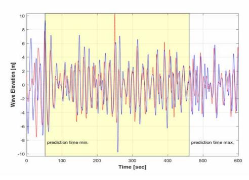
**Fig. 14** Comparison between the predicted wave at gauge position #2 (blue line) based on the irregular wave measurements at gauge position #1 and the measured wave at gauge position #2 (red line) under condition1-seed#1
