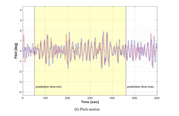
**Fig. 17** Motion prediction based on wave information at gauge position #1 under head sea/condition 1/random seed #1 with (a) heave, and (b) pitch motion. The red dashed line depicts the result of motion prediction and the blue dashed line depicts the measured motion.
