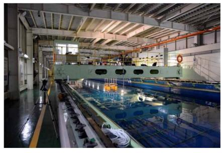
Fig. 2 Photo of the towing carriage with the TLP model
