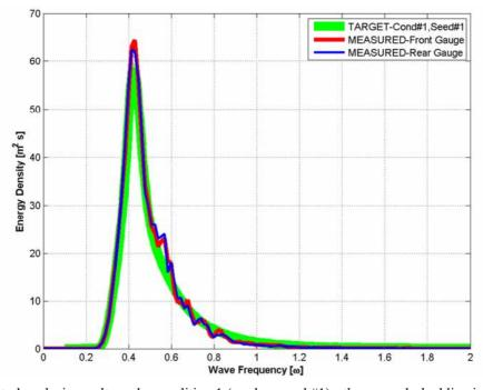
**Fig. 13** Spectral analysis results under condition 1 (random seed #1) - the green dashed line is the input wave condition, the red dotted line is the wave spectrum of its irregular wave at gauge position #1, and the blue dotted line is the wave spectrum of its irregular wave at gauge position #2.
