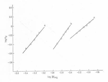
Figure 1. Plot of  $\log K_d$  vs.  $\log [B]_{org}$  for the extraction of Mn(II) with 10 mM BMPP in benzene. [B]\_{org} represents (a) 4-methyl pyridine N-oxide (pH = 5.70) (b) pyridine N-oxide (pH = 5.60) (c) 2-methyl pyridine N-oxide (pH = 5.60).
