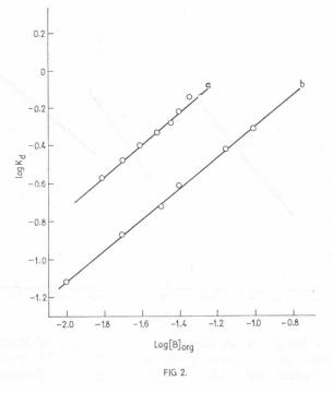
Figure 2. Plot of  $\log K_d$  *vs.*  $\log [B]_{org}$  for the extraction of Mn(II) with 10 mM BMPP in benzene. [B]<sub>org</sub> represents (a) dibenzylsulfoxide (pH = 5.0) (b) 8-aminoquinoline (pH = 5.50).
