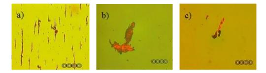
**Figure 4.** The demonstration of particles trapped onto the ferrograms of oil samples **Slika 4.** Prikaz čestica u uzorku ulja uhvaćenih ferogramom
